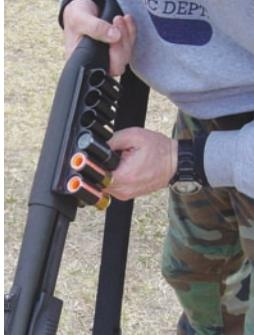
The shell carrier on this 12-gauge is filled with several different types of non-lethal ammo.
